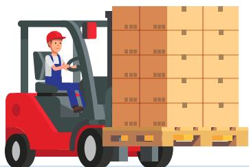
This is the most widely used type of forklift, characterized by its counterweight at the rear to maintain stability while lifting and moving loads. It's versatile and suitable for various applications in warehouses, industries, retail distribution centers, and more.
